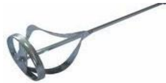
WRONG Paint Mixing Blade:
